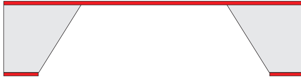
Figure 3.5: Illustration of the SiN membrane structure
